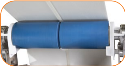
STANDARD FEATURE: V-Guided Belt Tracking
