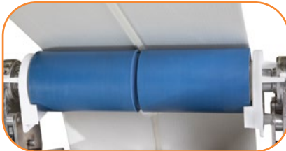
STANDARD FEATURE: V-Guided Belt Tracking
