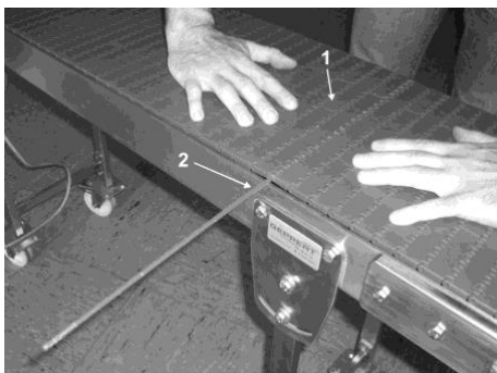
Figure 4-8: Opening and closing the conveyor chain
