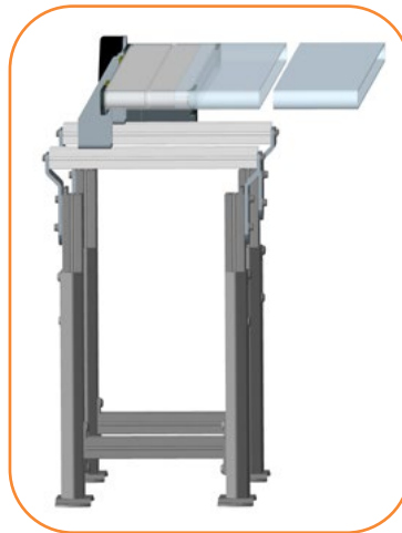
Easy Access for Quick Belt Removal
