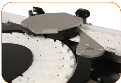
Divert Module with Sensors
