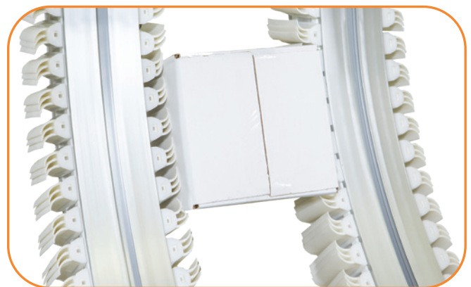
Products are wedged between opposing conveyors
