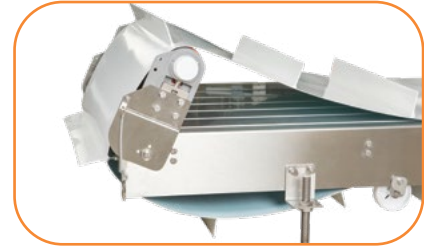
STANDARD FEATURE: Tip-Up Tail**
