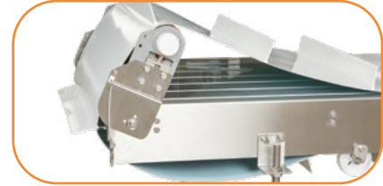
STANDARD FEATURE: Tip-Up Tail**
