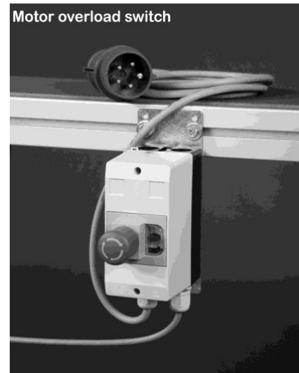
Figure 3-5: Motor overload switch
