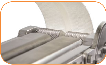
STANDARD FEATURE: V-Guided Belt Tracking
