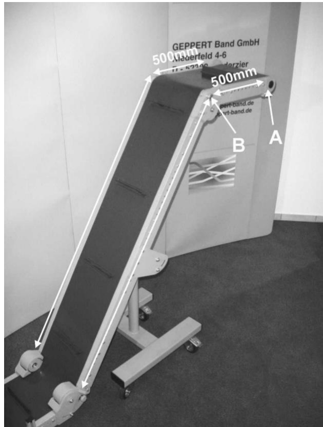
Figure 4-13: Axial distances on Z-shaped belt conveyor
