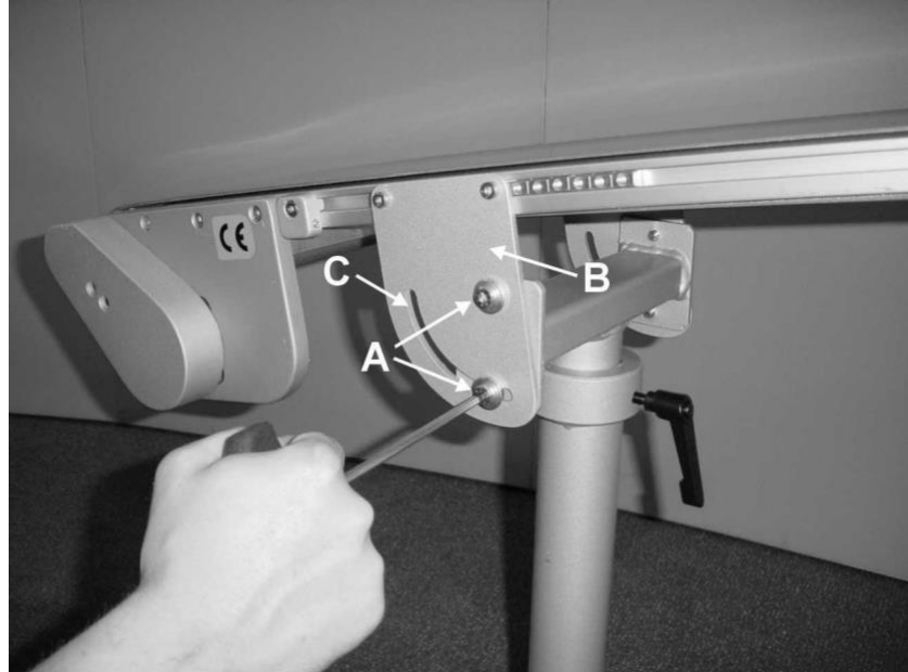
Figure 4-22: Single-legged steel support with aluminium base plate, inclination adjustment
