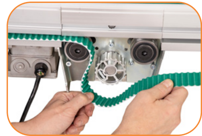
STANDARD FEATURE: Quick belt change without the removal of conveyor or accessories
