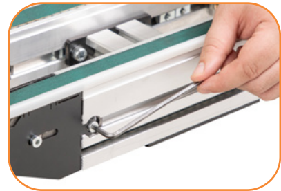
STANDARD FEATURE: Tensioning Mechanism
