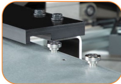
STANDARD FEATURE: Pin Tracking Bearing Cams smoothly guide the pallets around corner
