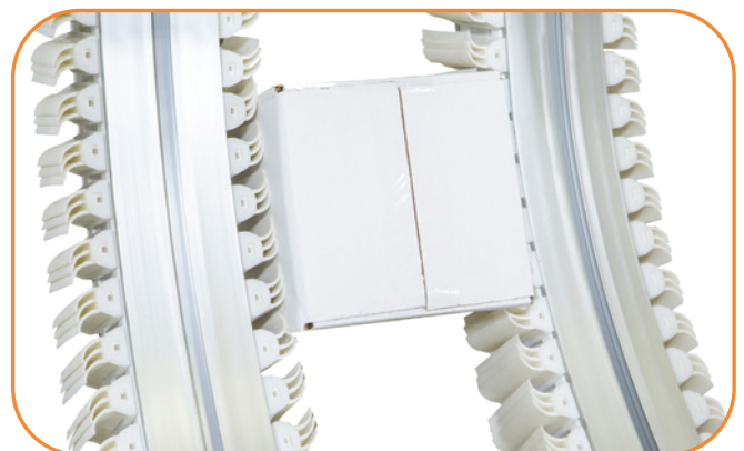
Products are wedged between opposing conveyors
