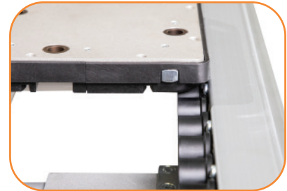
STANDARD FEATURE: Conveyor roller provides pallet guiding
