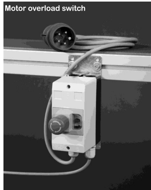
Figure 3-7: Motor overload switch
